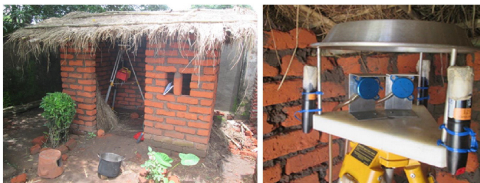
Fig. 2. Test kitchen and monitoring equipment.
