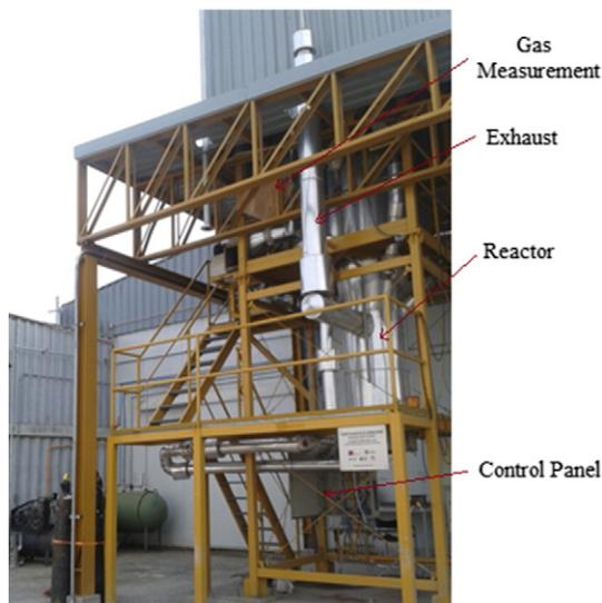
Fig. 4. Cofiring plant installed at UDT (University of Concepción).
