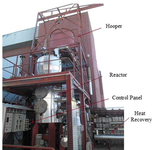
Fig. 3. Torrefaction plant installed at UDT (University of Concepción).
