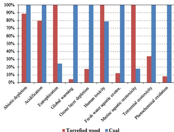
**Fig. 5.** Characterized results from the coal and torrefied biomass. CML 2 Baseline 2000 v2.05/World 1995.
