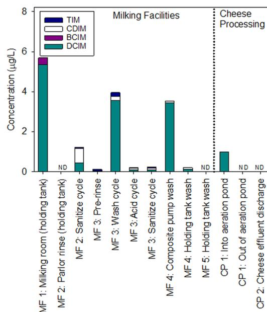
**Figure 2.** Concentrations of iodo-THMs in water from various spatial locations within the dairy processing cycle at five milking (MF 1–5) and two cheese processing facilities (CP 1–2). Abbreviations: DCIM, dichloriodomethane; BCIM, bromochloriodomethane; CDIM, chlorodiiodomethane; TIM, iodoform.
