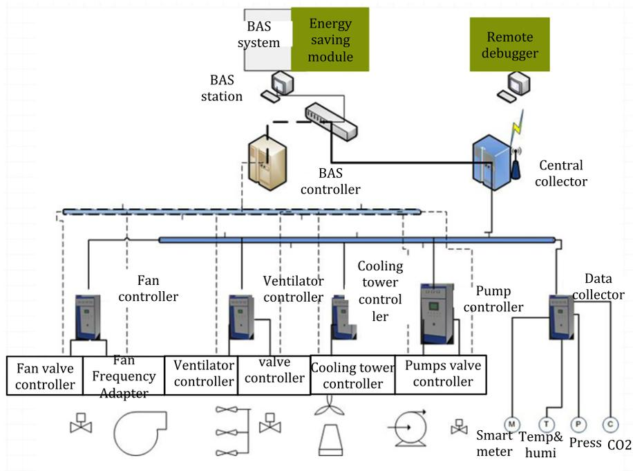
Fig. 9. System architecture of autonomous HVAC control systems.
