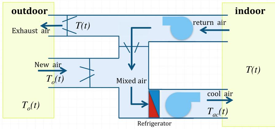
Fig. 5. Air flow in the subway HVAC system.
