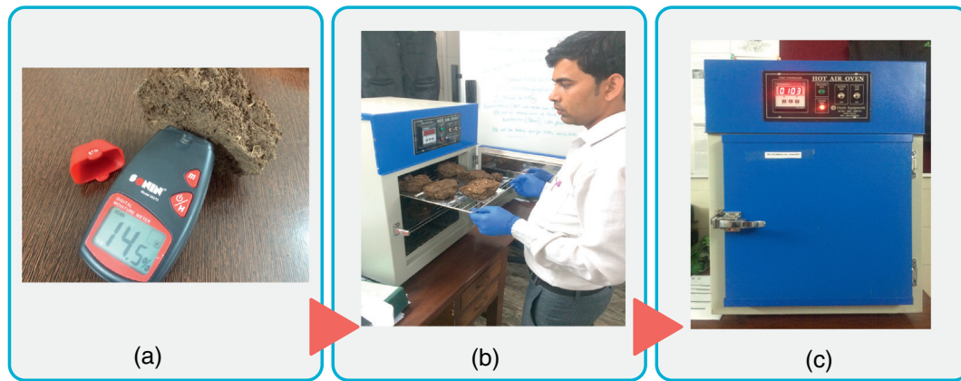
Fig. 3. Moisture measurements: (a) moisture meter with sample, (b) sample arrangement in convection oven and (c) convection oven.
