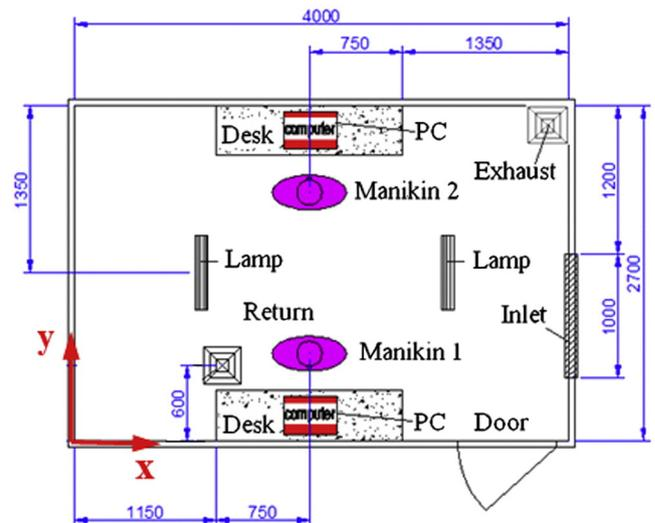
Fig. 5. The arrangements of the climate chamber.
