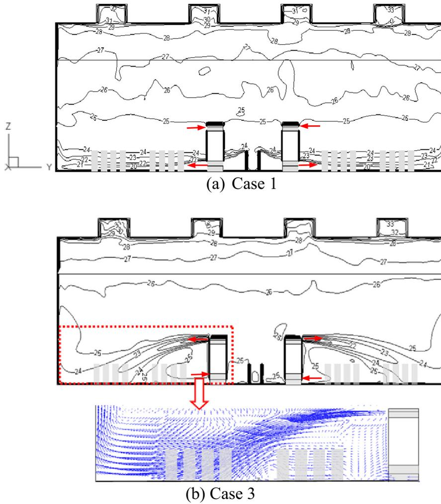
Fig. 7. The temperature and velocity distributions at Plane X = 5.6 m in Case 1 and Case 3.
