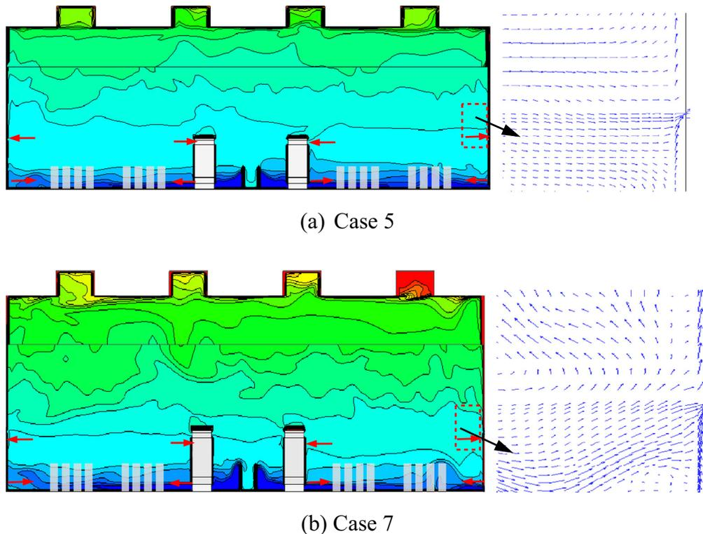
**Fig. 11.** Temperature contours and local velocity vectors at Plane X = 5.6 m in Case 5 and Case 7.
