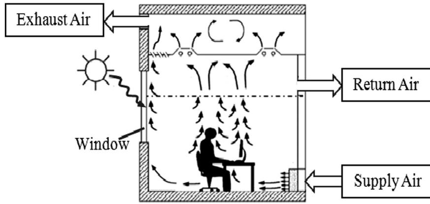
Fig. 2. A stratified air distribution system with separate locations of return and exhaust grilles.
