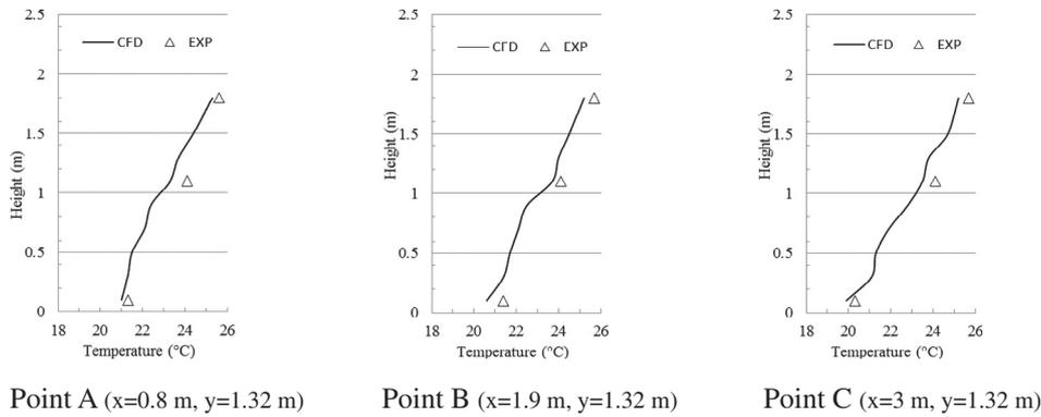
Fig. 6. Comparison of simulated and measured temperature profiles.
